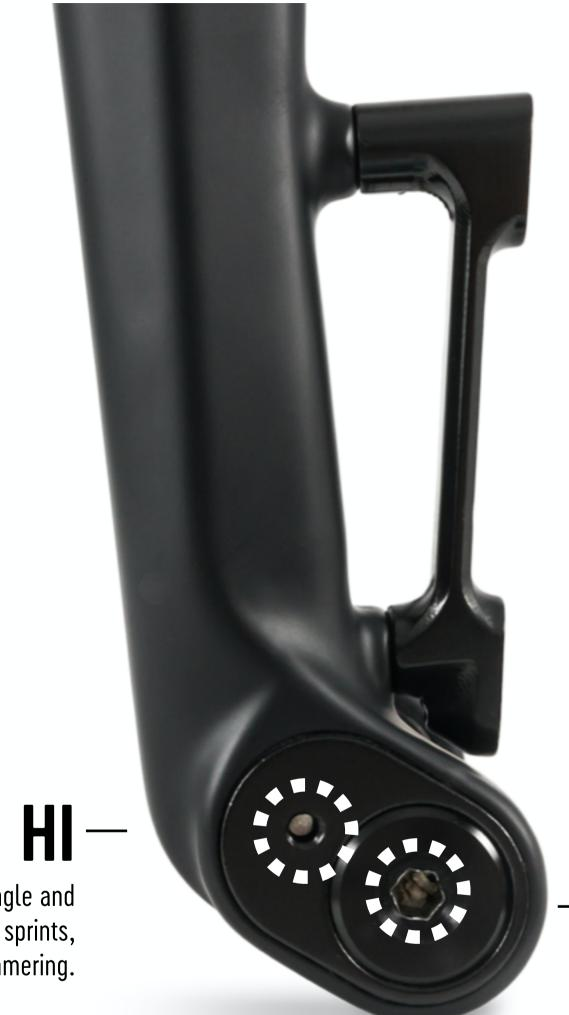
This position gives the bike a higher front end, slacker head angle and longer trail Ideal for comfortable long distance riding.
